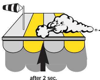
As long as the measured wind speed is higher than the adjusted threshold, any order is inhibited.
